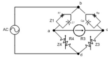
$$\frac{1}{Z_1} = \frac{1}{R_1} + \frac{1}{1/j\omega C_1} = \frac{1}{R_1} + j\omega C_1$$
