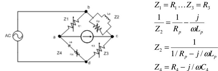
$$R_1 R_3 = \frac{R_4 - j/\omega C_4}{1/R_p - j/\omega L_p} \quad \frac{R_1 R_3}{R_p} - j \frac{R_1 R_3}{\omega L_p} = R_s - j \frac{1}{\omega C_4}$$
